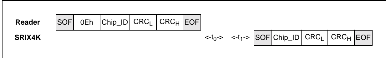
Figure 25. SELECT Frame exchange between Reader and SRIX4K
